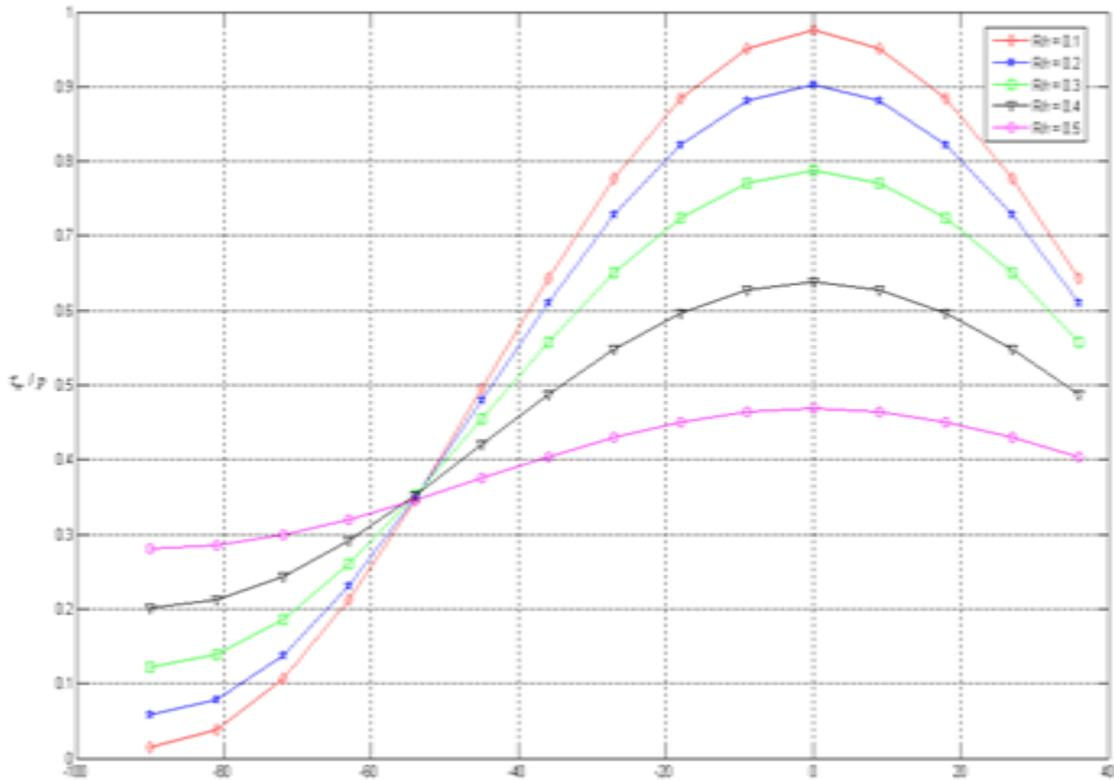
Fig. 2 Distribution of the Stress Component  $\tau_{rr}$  Round the Edge of a Circular Hole
