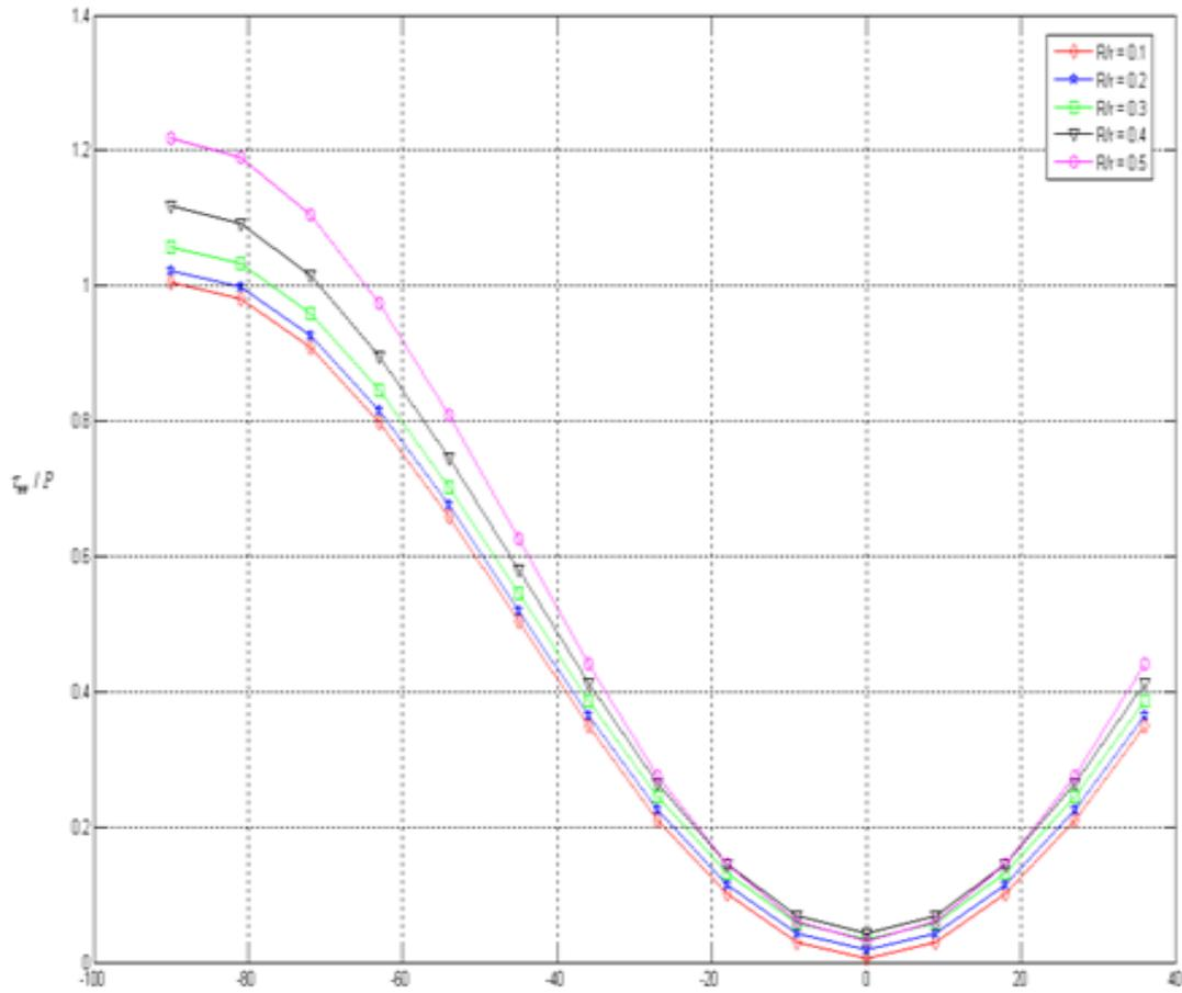
Fig. 3 Distribution of the Stress Component  $\tau_{\theta\theta}$  Round the Edge of a Circular Hole
