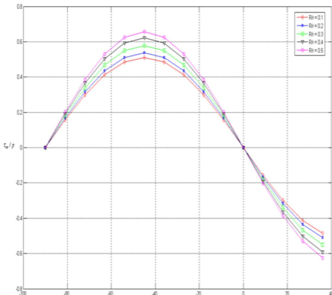
Fig. 4 Distribution of the Stress Component  $\tau_{r\theta}$  Round the Edge of a Circular Hole
